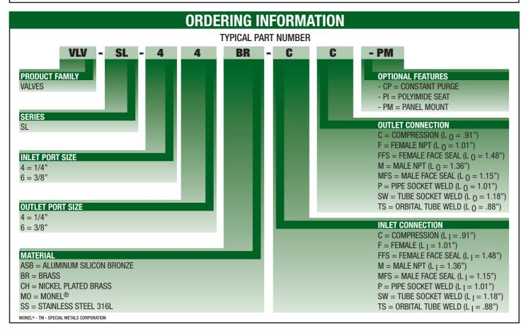
3 PORT, 4 PORT AND CUSTOM CONFIGURATIONS ARE AVAILABLE ON REQUEST. ALSO AVAILABLE WITH PNUEMATIC OPERATOR, SEE LPSL SERIES.
